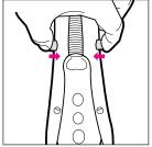
Press Handheld release buttons inward to release Handheld unit.
